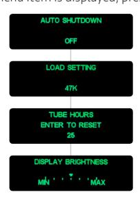
'OPTION' on the front panel or remote to adjust the settings of that particular selecton. After making the appropriate change, pressing the 'ENTER' button will confirm the new setting, and the display will show 'OKAY' for five seconds before reverting back to the normal operation screen.
