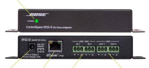
**12VDC input:** +12VDC @ 500mA, center-positive polarity (External supply not required if used with a PoE Ethernet switch)
