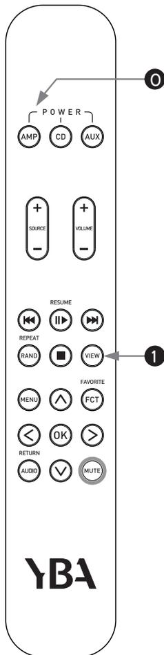
**0** Select the device you want to control between AMP, CD and AUX. To control the A6, you need to select AMP button.
