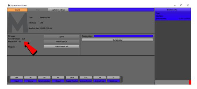
The firmware can be updated by using USB2 port and Mytek Control Panel application. It does not require installed USB2 driver (PC). To download the current firmware please visit: mytekdigital.com
