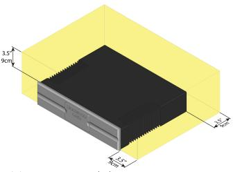
Minimum recommended clearance for heat dissipation
